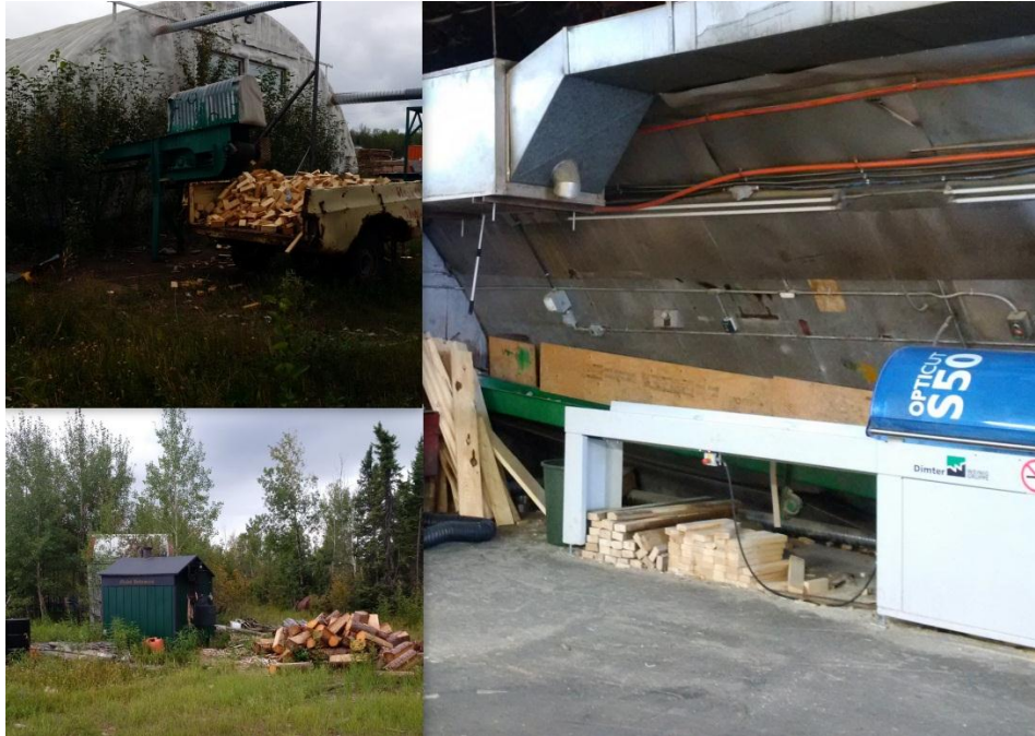
Figure 5. Trim saw equipped with conveyer (shown “green”) to move ends to exterior dump trailer for end use in outdoor wood furnace (Note: no preserved wood is used in process).
