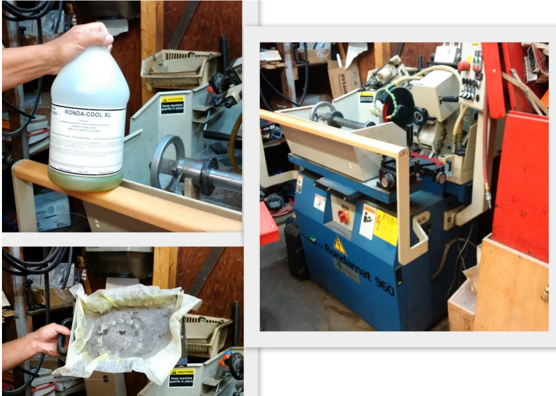
Figure 7: Rondamat 960 sharpener with screen collection system for filings from moulder bits. Ronda- Cool XL grinding lubricant is recycled within system.
