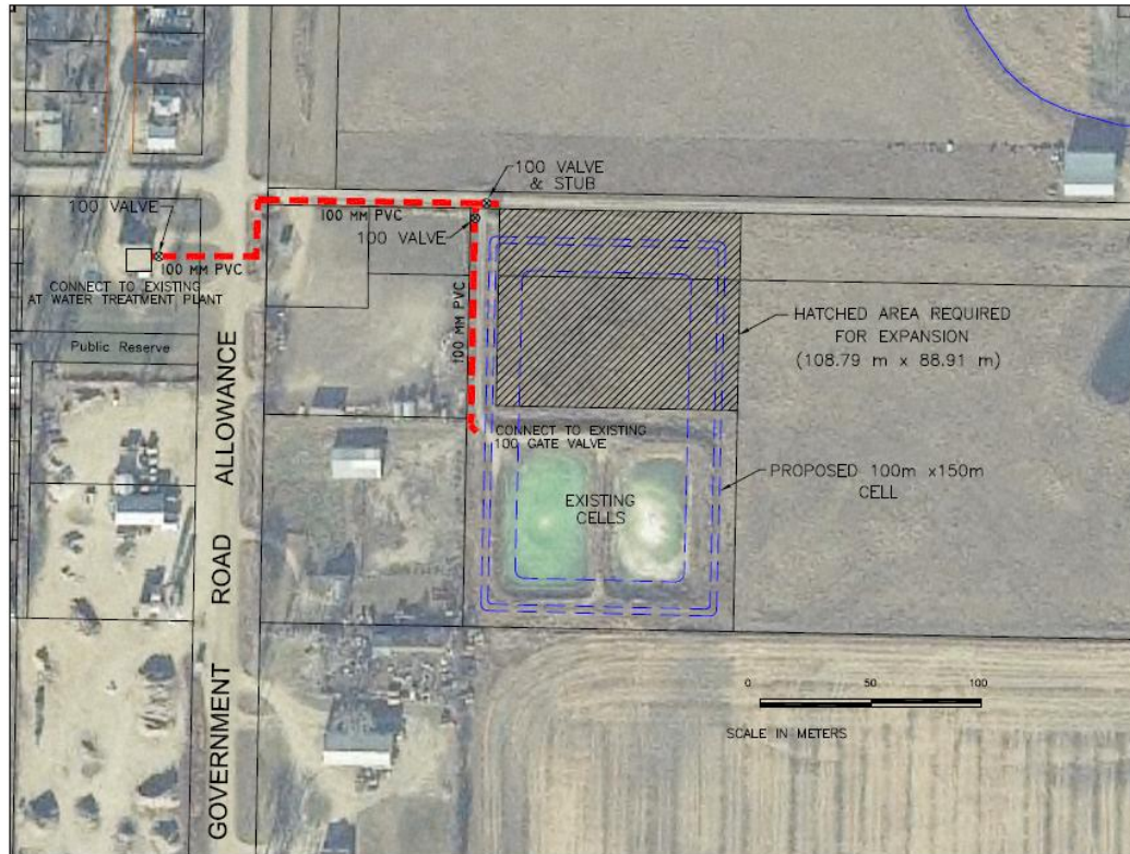
FIGURE 2.2 – EXPANSION OF REJECT WATER STORAGE CELL
