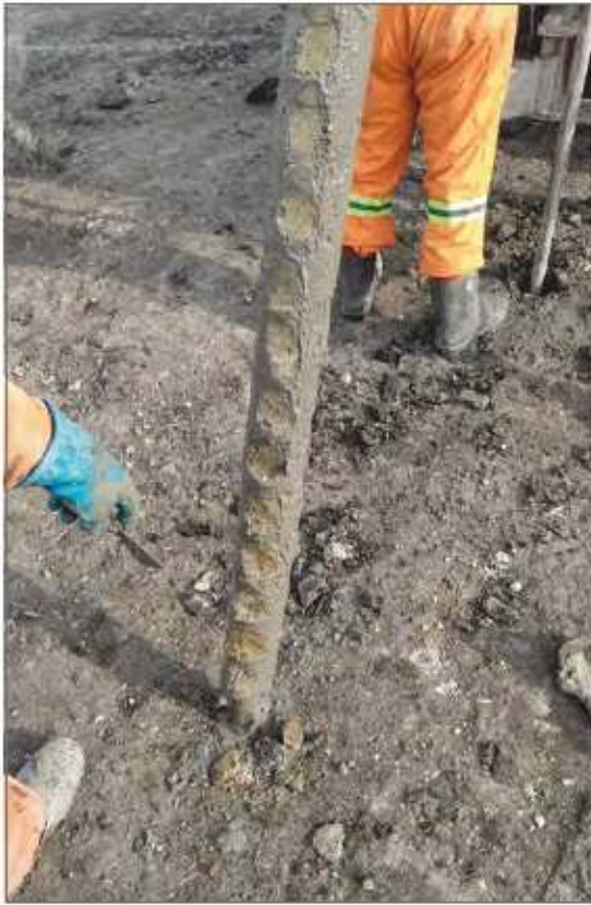
Photo 1: Clay Till Material in Borehole 22BH01
