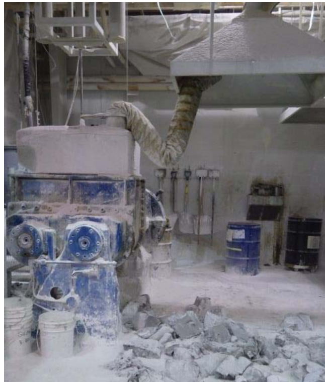
Photo 24. Sealants mixer and sealant prior to extrusion.
