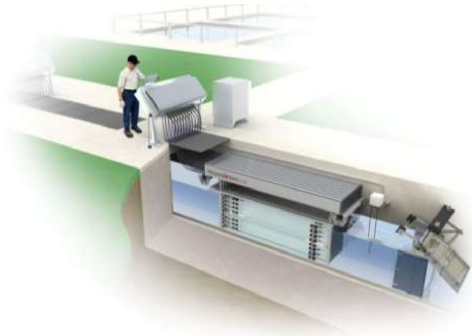
Figure 3.8: UV Installation in Channel (Image from Trojan UV)
