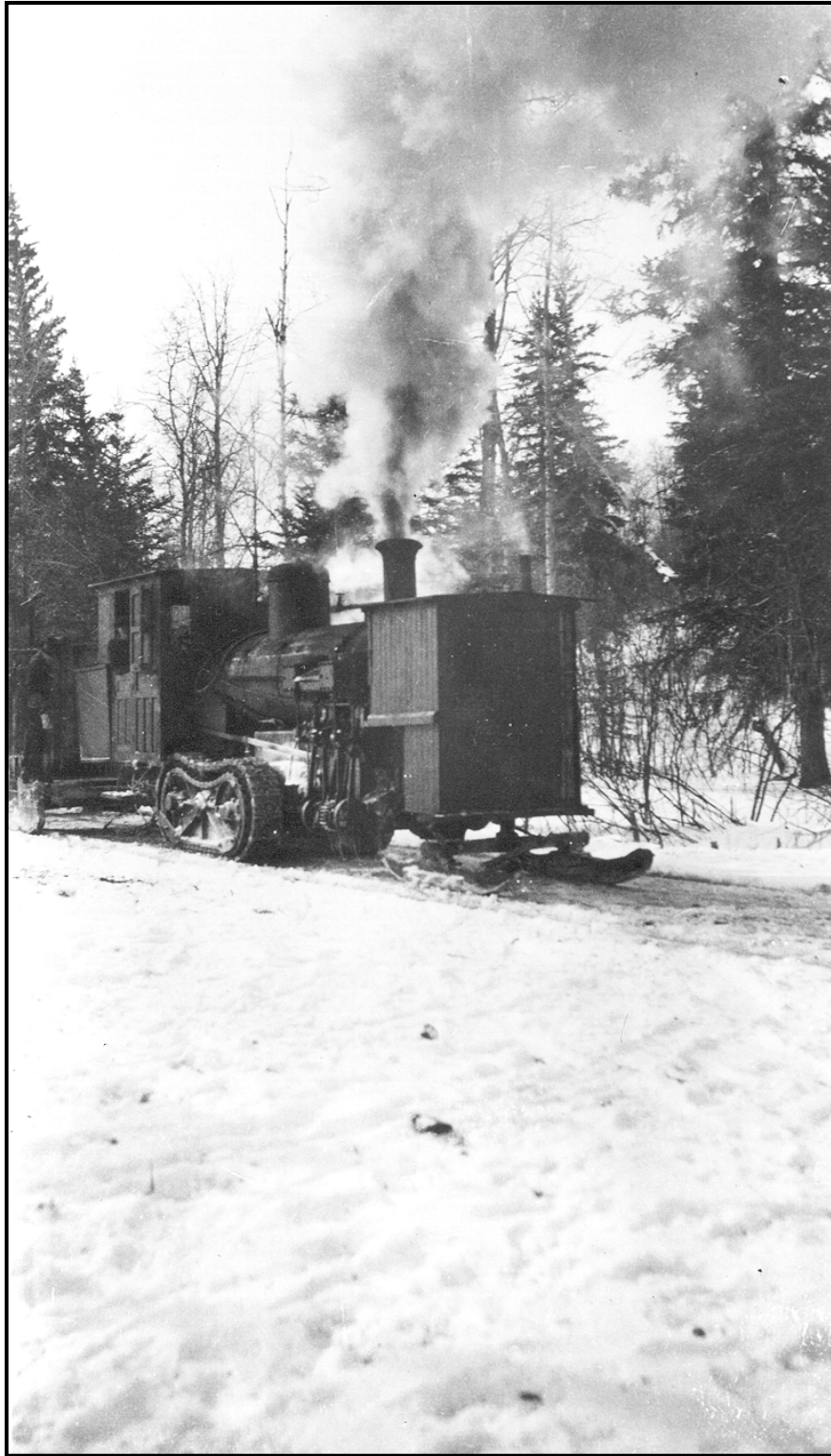
A steam log hauler in use in the Duck Mountains, 1919. Source: P.A.M.
