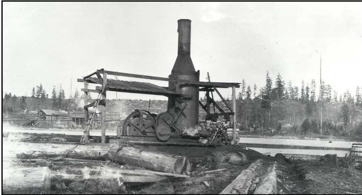
A steam engine used to provide the power for a sawmill at Manigotagan, c. 1904-1915 Source: P.A.M.
