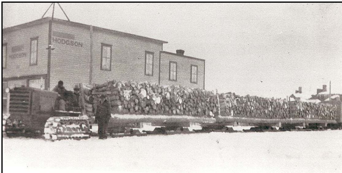
A cat train hauling cordwood from the Lake St. George area to the railway at Hodgson, 1938. Source: P.A.M.
