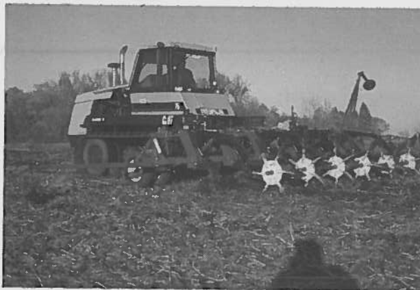
Figure 3.4-7 Fall bedding and reservoir tillage implement (Courtesy of Gaia Consulting Limited)
